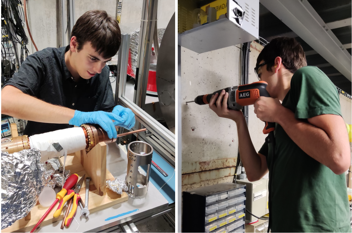
Figure 11: Screwing of the BASE trapcan indium flange and drilling mounting holes for the medicine cabinet
